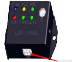
LED control panel
